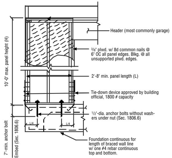
Figure 6—Alternate braced wall panel, one-story building.
