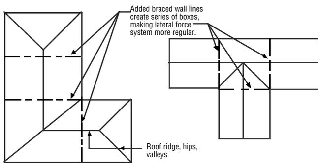
Figure 3—T- and L-shaped buildings. Added braced wall lines provide conventional “box” bracing system.
