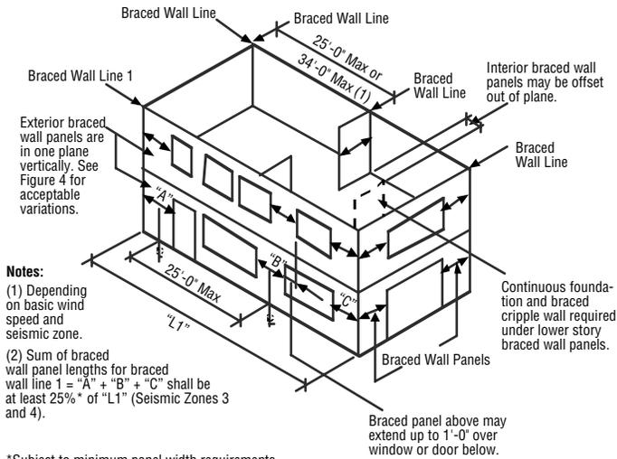
Figure 2—Acceptable bracing example—two-story building.
