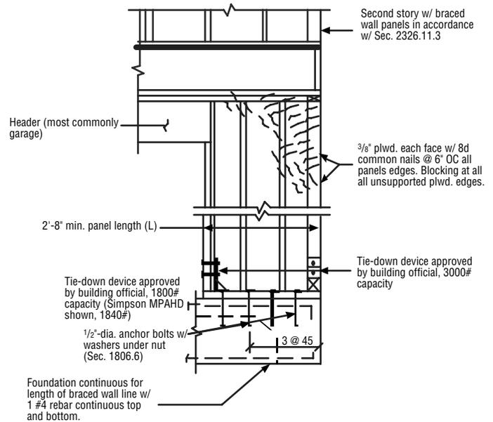
Figure 7—Alternate braced wall panel, first story of two-story building.
