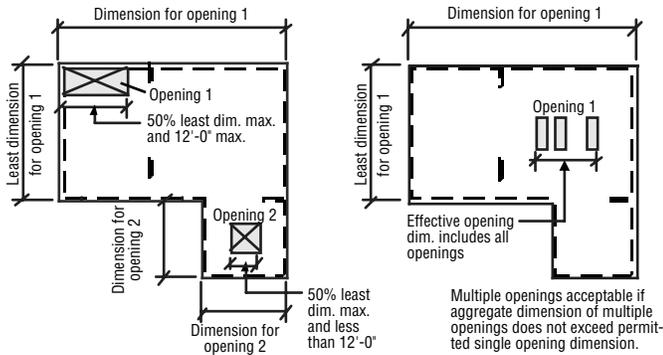
Figure 5—Acceptable floor and roof openings.
