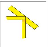
Figure 2 Typical rafter and ceiling joist connection with no soffit at eave.
